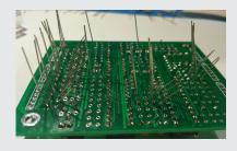
After stuffing a group of resistors, I bend the short leg at an angle to hold the resistors onto the board.
