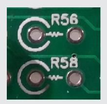
The resistor silkscreen has a circle where the base (tolerance band) is placed and a small resistor symbol pointing toward the associated pad for the bent lead.
