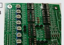
Insert Trim pots R16-R22. Verify the proper value of each before installing. Ensure that the trim pot Pin 1 is inserted into
