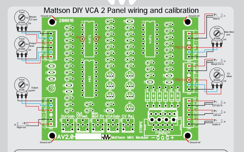
Qty 6, TS Jacks, switched, Normally closed. J1-J6 Panel components required: Qty 4, B100K Potentiometers (Linear).
