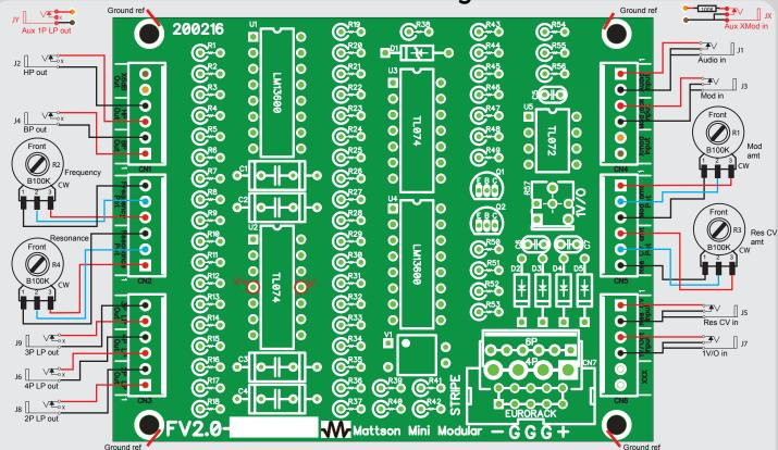
DIY builder note: JX can be installed to CN4-5,6 for an eXtra mod input. JY can be used on CN1-5,6 for a 1P, 3dB LP output if desired.
